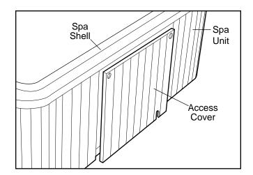
To replace the access cover, insert the bottom of the cover into the slot of the spa shell. Firmly push the top closed.
